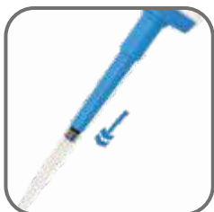
Eject Tips Easily with a Tip Ejector
